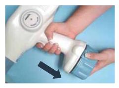
3 Carefully insert a newly charged battery into the base of the NOMAD handle (a properly oriented battery should click into place without force, forcing the battery into position may damage the battery and/or the NOMAD). A clicking sound ensures that the snaps on both sides of the handle bottom are fastened. Make sure the battery is secure by giving it a tug. When a battery is detached, any stored exposure time is erased from memory and has to be reset when the unit is turned on again.
