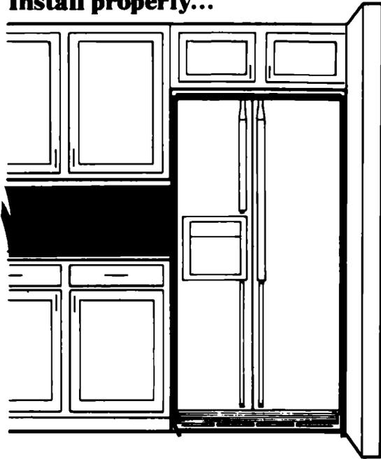
1. Allow ½ inch (1.25 cm) space on each side and at the top of the refrigerator for ease of installation.
