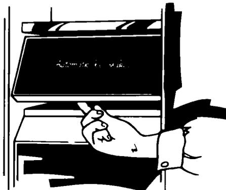
1. Pull the covering panel out from the bottom and slide it to the rear.
