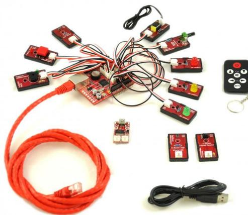
The kit doesn't come with a processor board giving the user further flexibility selecting a device. FEZ Domino, FEZ Panda or FEZ Panda II are ideal mates for the Internet of Things Kit. The kit even works with Arduino and its derivatives, keeping in mind that all open-source code samples in this book are aimed to using C# for FEZ and .NET Micro Framework.
