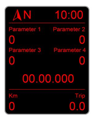
As can be seen in the picture, in the top of the screen, the first 4 parameters of the active desktop are shown, and in the bottom, the stopwatch time is indicated. If there is any key configured to switch desktop, it will change the desktop displayed.
