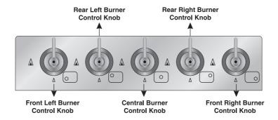
**Use the front left and the front right burners** for simmering or for cooking smaller quantities of food requiring small cookware.
