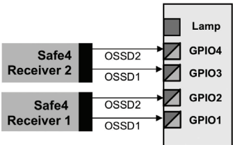
Figure 10: Connection of up to two OSSD safety components (e.g. GuardShield Safe4 light curtain systems)
