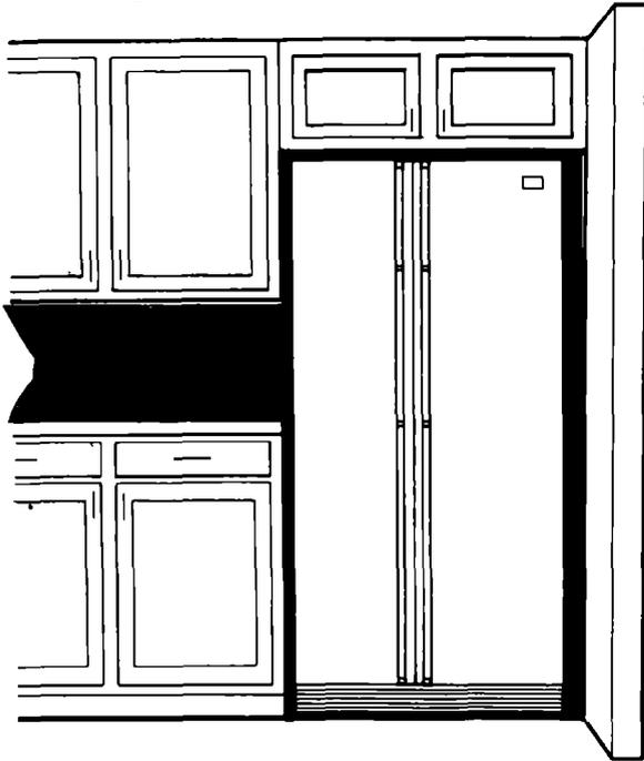
1. Allow ½ inch (1.25 cm) space on each side and at the top of the refrigerator for ease of installation.
