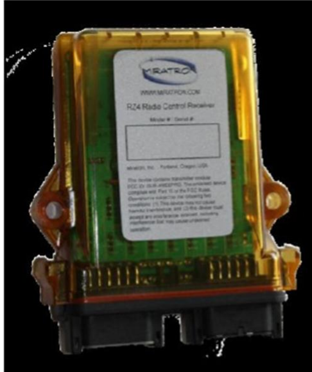
Figure 15: R-4 Programmable Remote Receiver Kill Switch.
