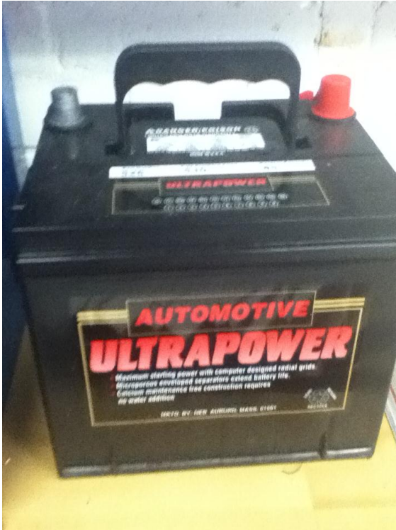
Figure 35: Centennial BCI Group 26 Sealed 12V Automotive Battery 550CCA.
