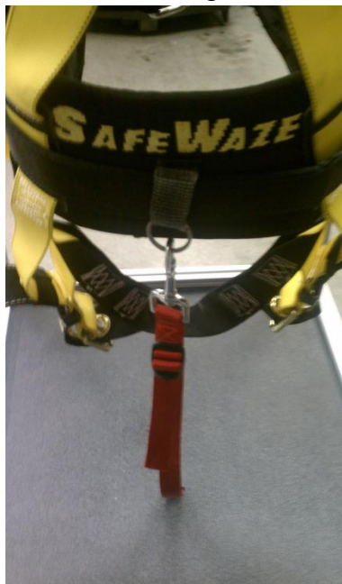
Figure 54: Safety strap attached to harness through top platform.
