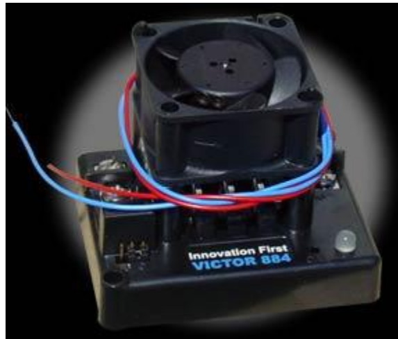
Figure 23: VEX Pro Victor 884 Speed Controller.
