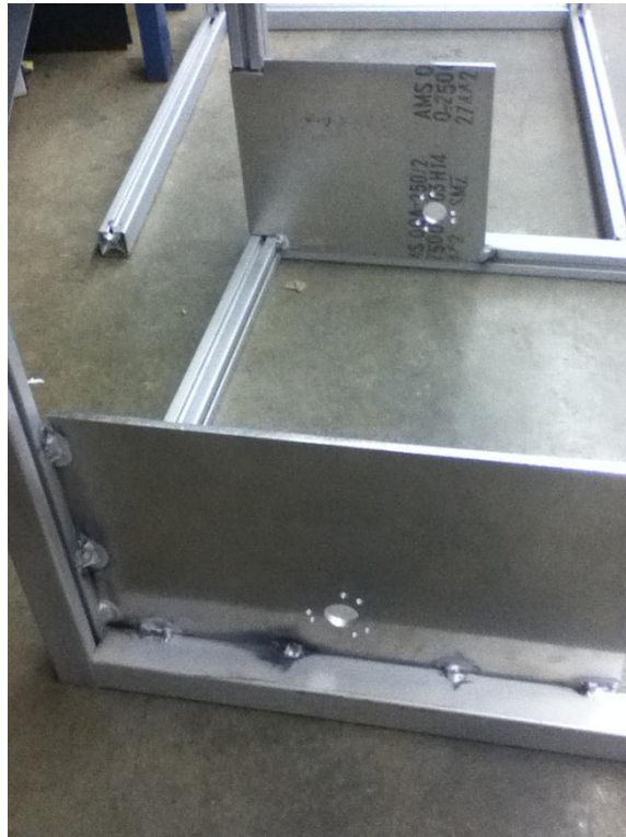
Figure 38: Plates after welding to the frame.
