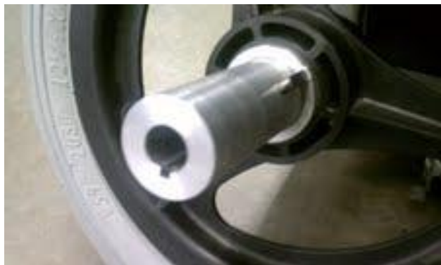
Figure 44: Coupler with inner and outer key slots.
