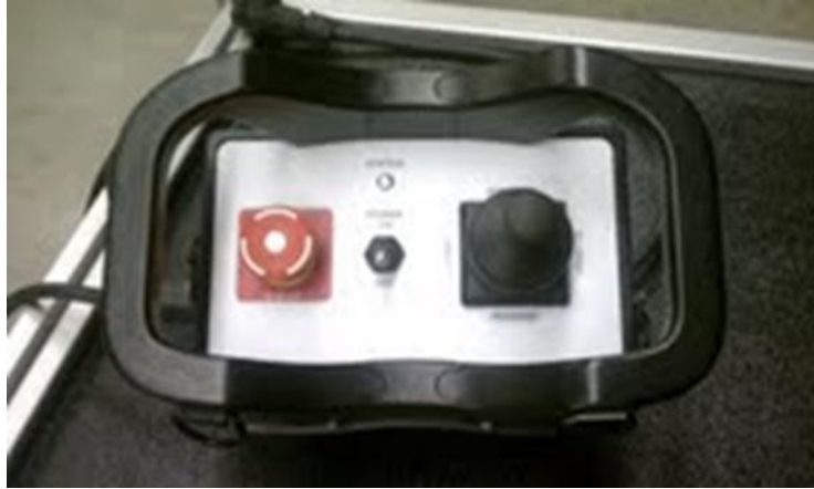
Figure 30: Parental control with emergency stop.
