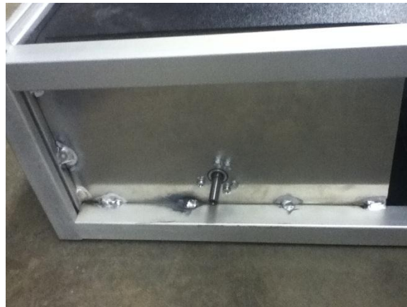
Figure 39: Motor mount with motor inside and top platform lowered above.
