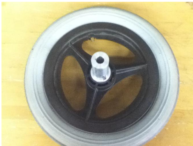
Figure 43: Inner view of wheel with coupler.
