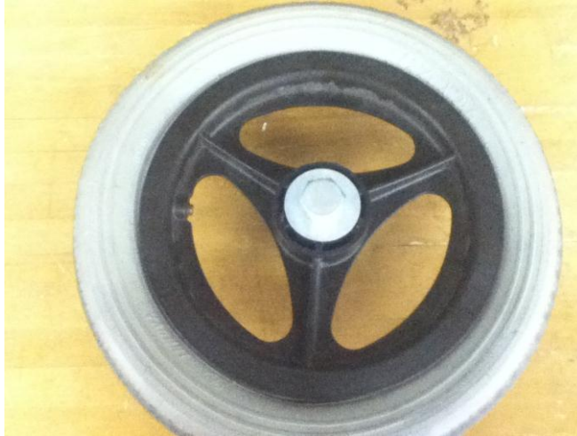
Figure 42: Outer view of wheel with large screw through to coupler.
