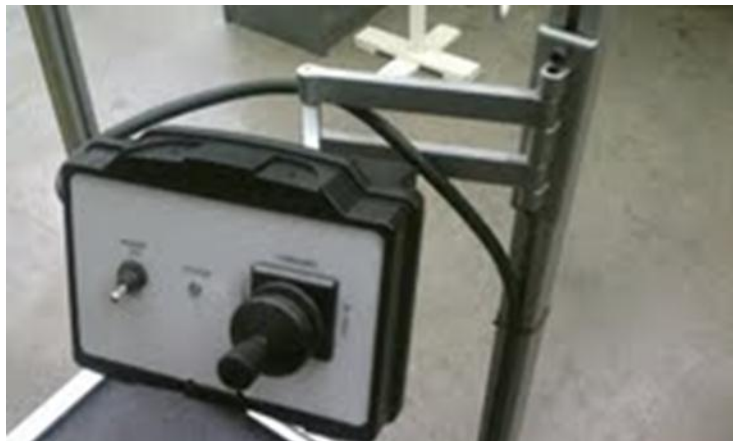
Figure 41: Control mount screwed into the 80/20 frame and attached to the transmitter.
