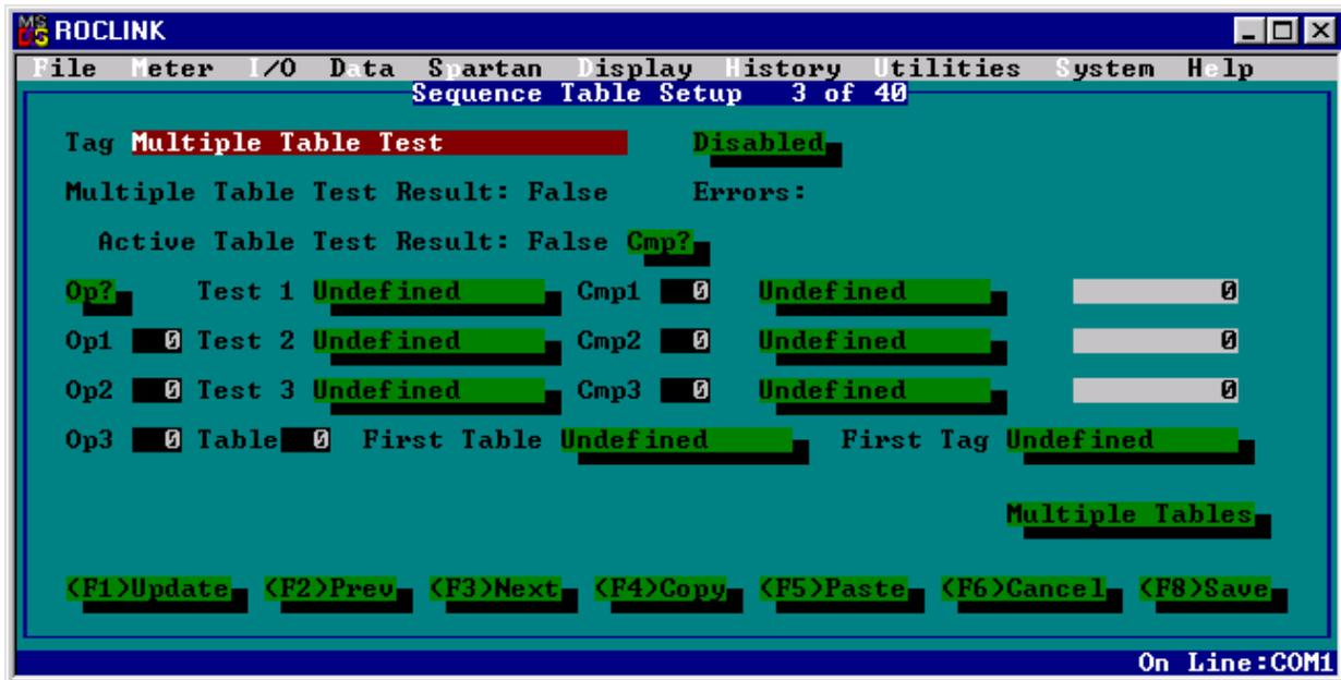
There are no tests configured on Table 3 (see Figure 3-7), but if the Multiple Table Test is true, the controls configured in the Multiple Tables will be executed.
