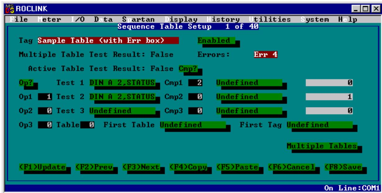
Figure 3-2 displays one of the Sequence Tables setup displays (1 of 40). All tests being performed are configured in these screens. There can be up to three parameters tested on each of the 40 sequence tables, and the tables can be cascaded.
