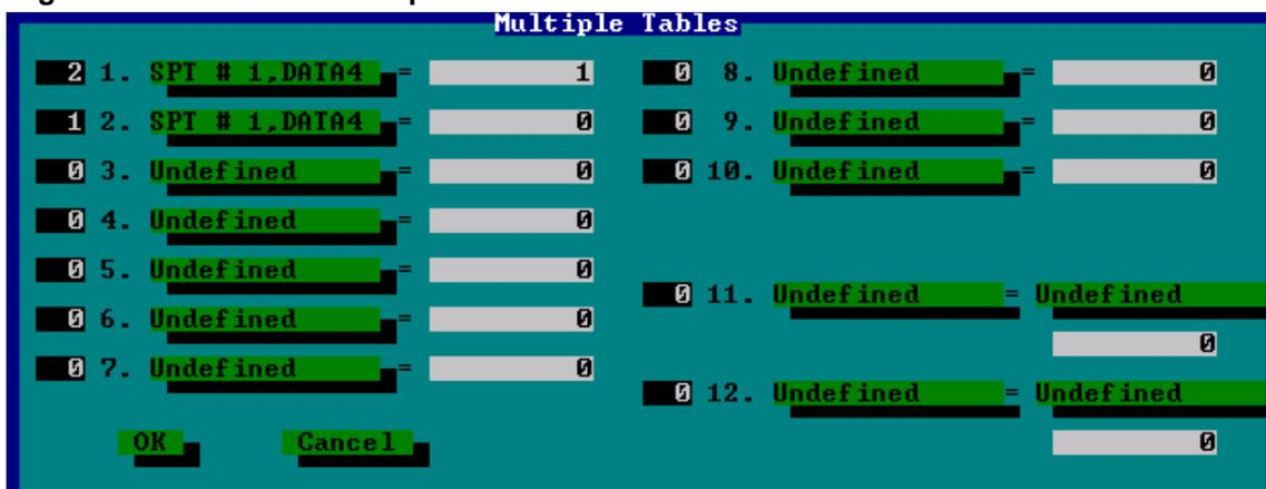
If the result of the Multiple Table Test is true, a value of 1 will be written to the Data4 parameter of Soft Point 1. If the result
