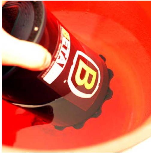
Figure 7: No continuous escaping air bubbles = 100% water-proof seal!
