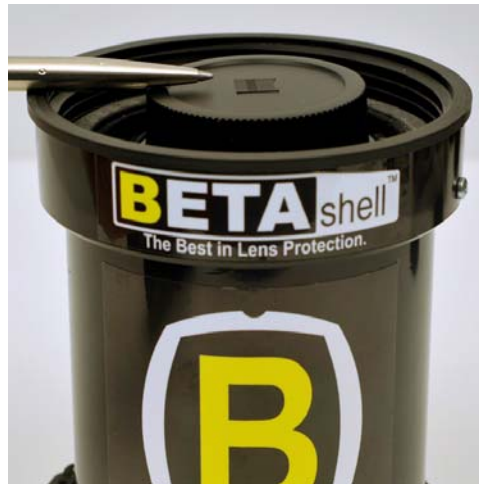
Figure 2: Limit of acceptable fit in lens case.
