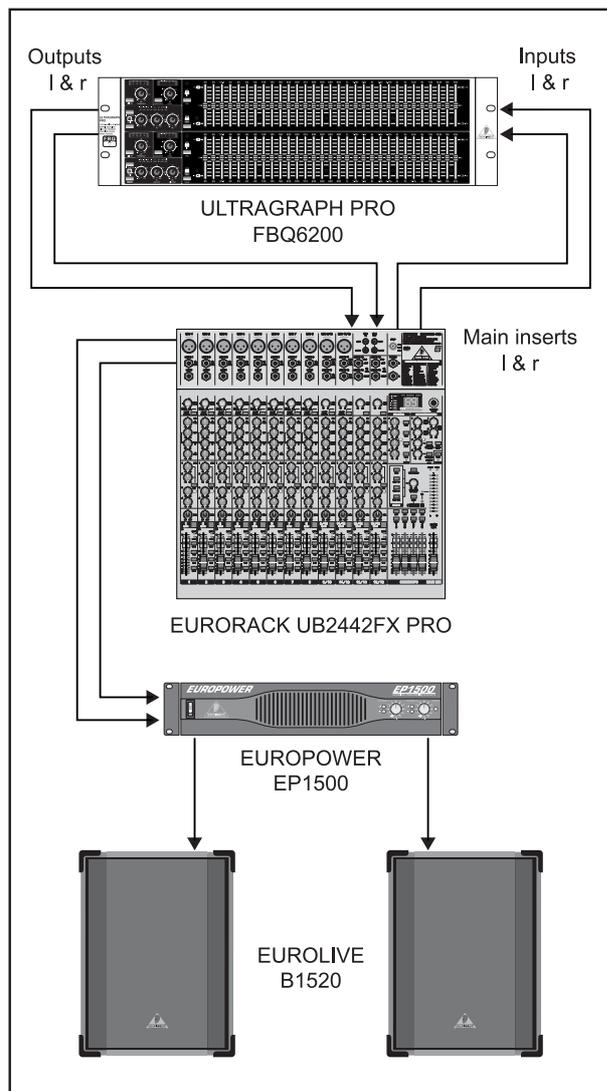
Fig. 3.1: The ULTRAGRAPH PRO FBQ6200 as master equalizer
