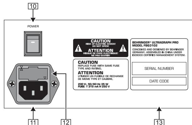
Fig. 2.2: Control elements and important information on the rear of the FBQ3102
