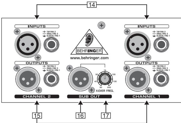
Fig. 2.3: Connectors at the rear of the FBQ3102
