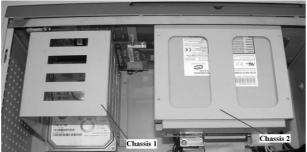
Fig 2-6.3 Chassis 1 and 2 for hard drive(s) installation
