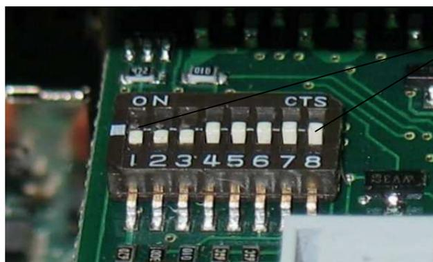
Fig. 34: DIP1-DIP8 switches (shown with factory settings)
