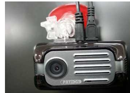
3. Mounted side or behind of mirror (※ careful tinted part of the windshield)
