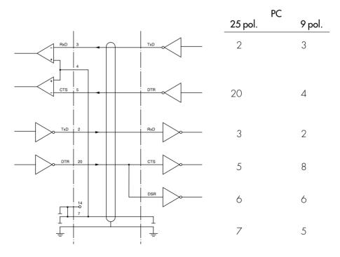
Type of cable: AWG 24 specification
