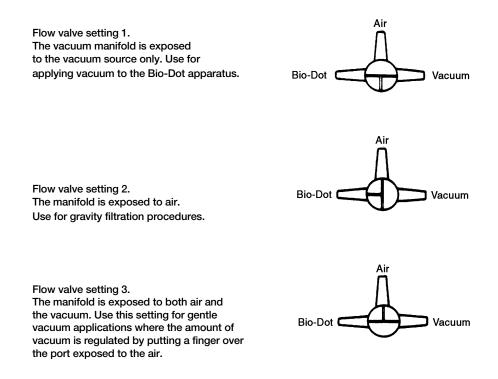
Fig. 3. Optional settings for the 3-way flow valve to obtain optimal performance from the Bio-Dot apparatus.
