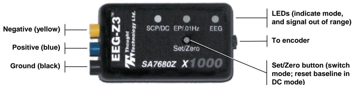
1. Connect the electrodes to the sensor using color-coded DIN cables. Respect the color coding as indicated in the preceding photograph.
