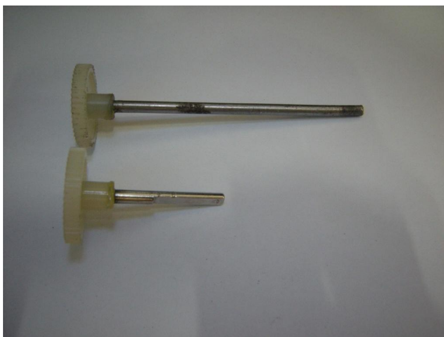
Figure 3.4: Original motor shaft and modified motor shaft
