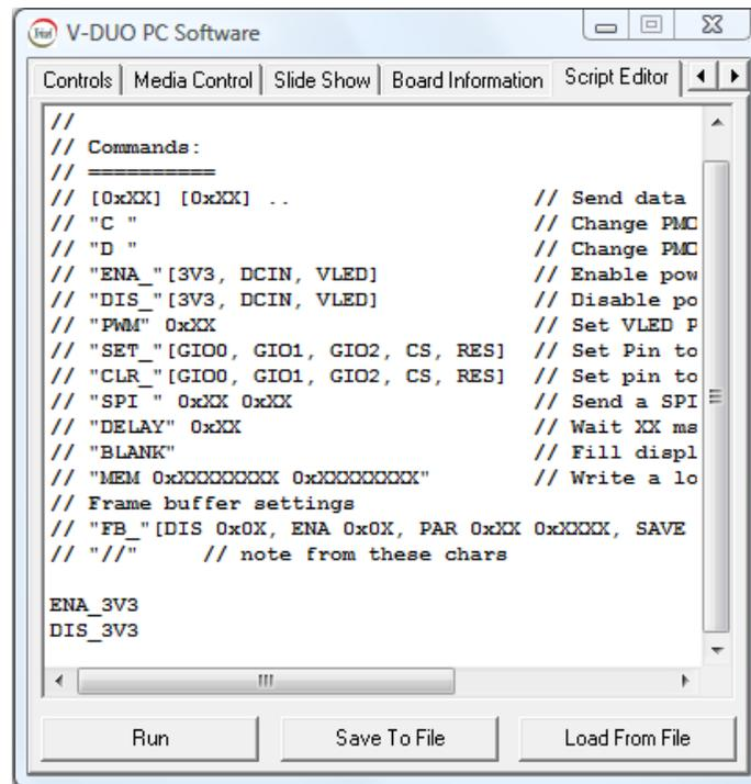
The DIS\_3V3 command will disable the 3V3 power supply and the screen will turn blank (white).
