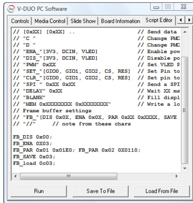
Framebuffer settings can be used to setup and select the following:
