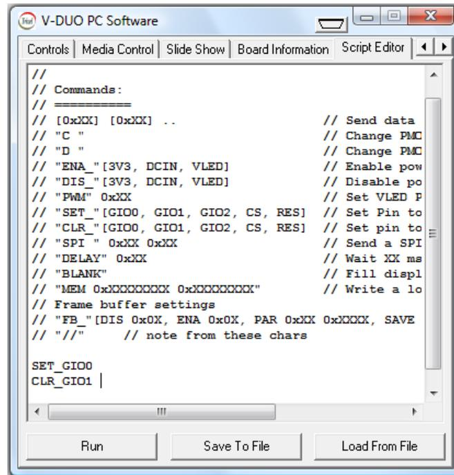
SET\_GIO0 will set the GIO0 pin. This command can also be used to set the GIO1, GIO2, CS and RES pins.
