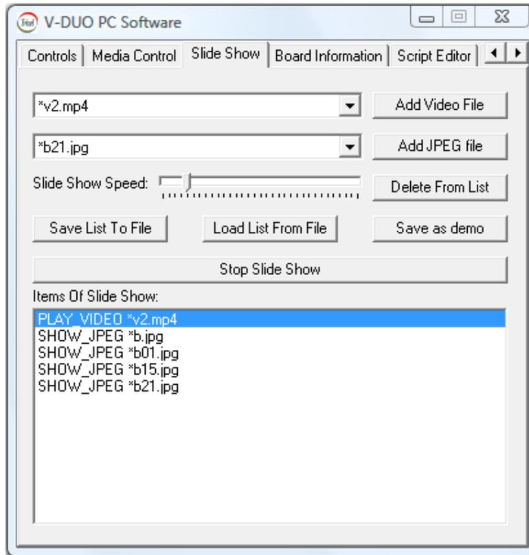
Video and JPEG files are added to the list of files to be shown in the demo by selecting the desired file in the drop down menu and clicking on 'Add video file' or 'Add JPEG file' respectively.
