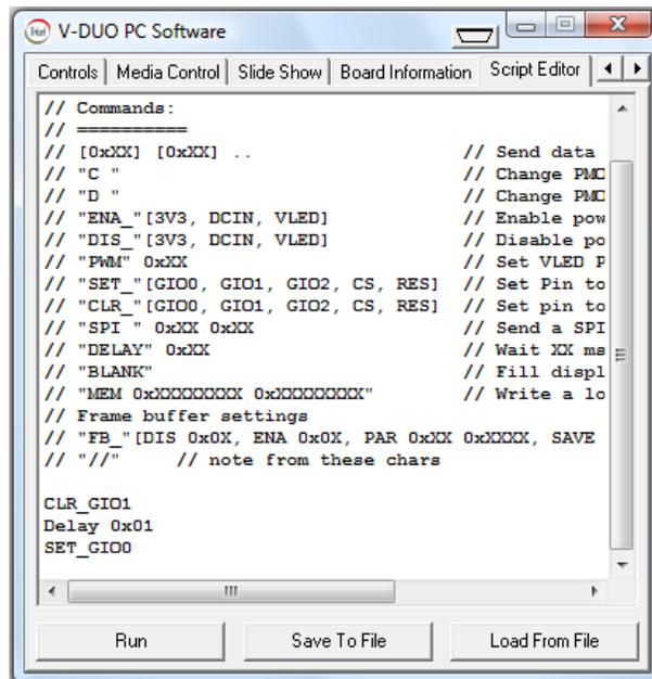
In the example on the previous page, the 'Delay 0x01' command will insert a time delay between executing the 'SET\_GIO0' command after executing the 'CLR\_GIO0' command.
