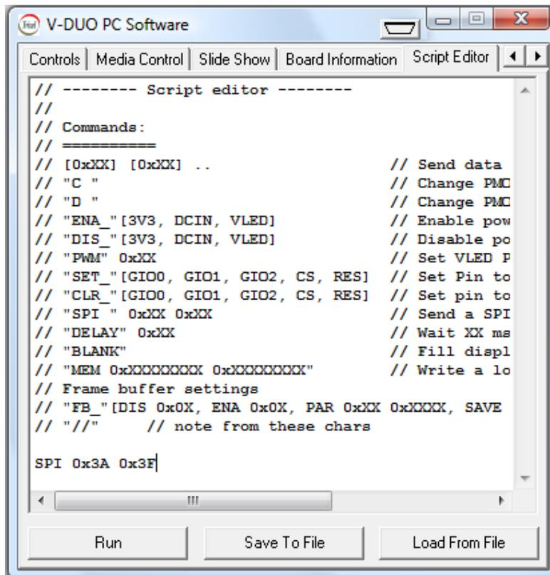
Referring to the image on the previous page, the SPI command is followed by the register address and the value to be written to it, both in hexadecimal. When the 'RUN' button is clicked, register 0x3A is assigned the hex value 3F (this is sent through the PIC microcontroller). This command will increase the overall contrast of the display to its maximum. Upon clicking the RUN button, the contrast change is immediately observed on the display.
