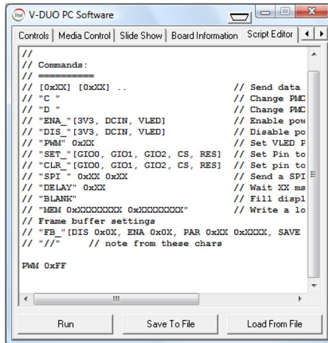
As shown above the PWM command controls the output voltage of the external DC-DC converter used for the High voltage supply (OLED\_VLED) on the PMOLED display interface.
