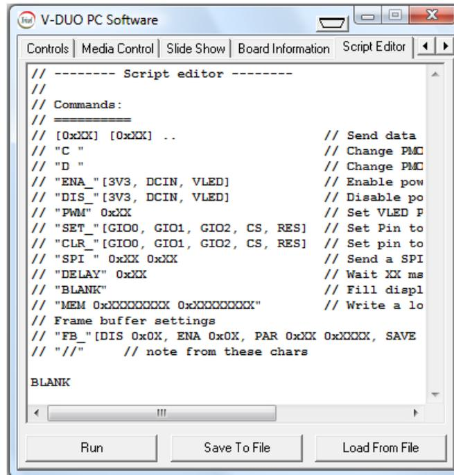
The BLANK command will turn the screen completely blank (with black screen). Basically it will clear the display buffers.
