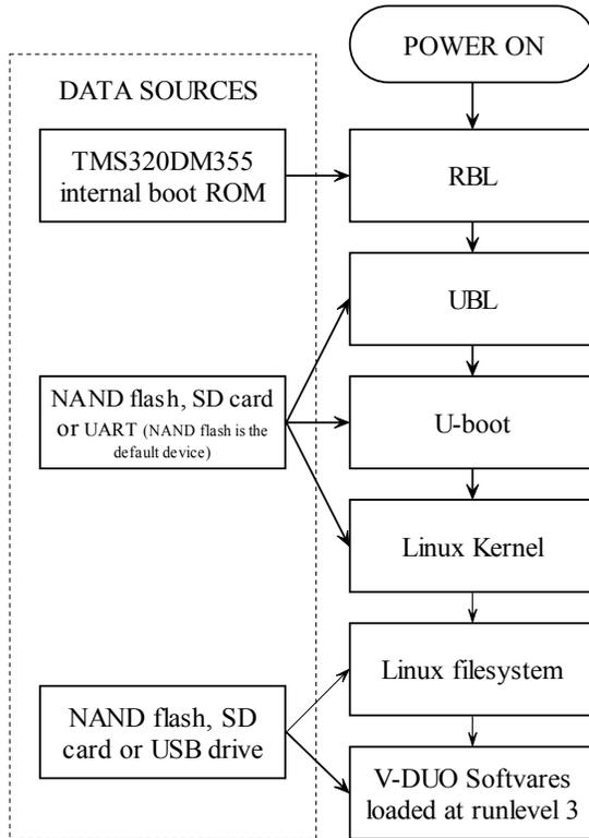
Alternatively, the system can boot from UART or SD card, as long as it contains the Linux style file system (EXT3) and the 'bootargs' settings are modified to boot from SD card (or UART). Please note that we do not recommend this operation unless the user has adequate experience, as the UBL and U-boot could be damaged.
