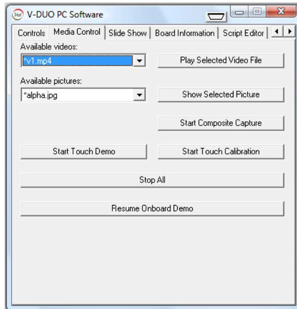
Clicking the 'Start composite Capture' button starts the capture of a valid composite video signal from the composite video input and displays it on the screen. If no composite video signal is detected or the format invalid, video capture will not start.
