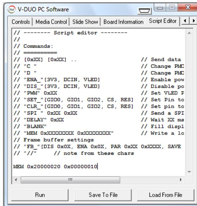
The 'MEM' command provides direct access to the V-DUOs internal system memory (NAND). With this command, any internal memory address in V-DUO can be written to. Misuse could overwrite or corrupt system files.
