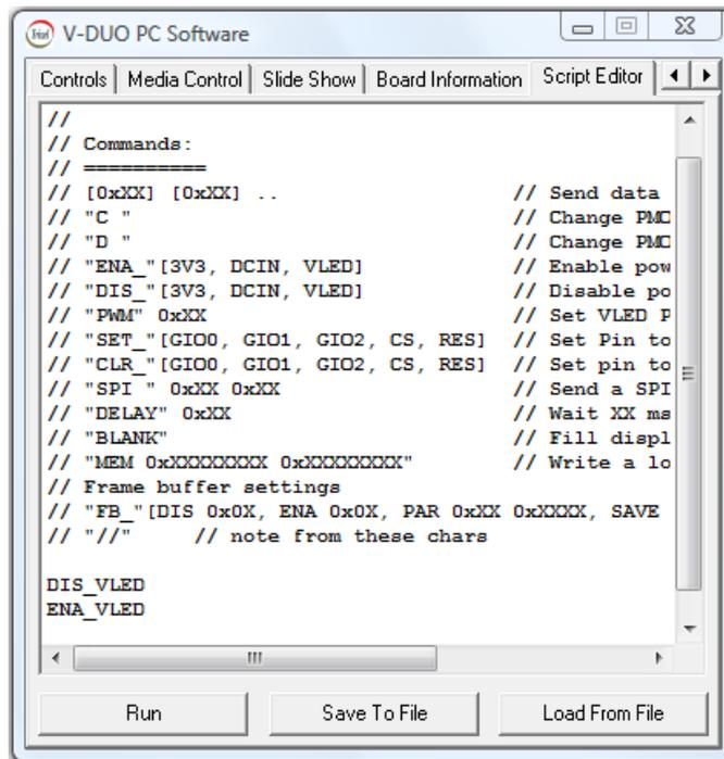
The DIS\_VLED command will disable the VLED power supply (external DC-DC). To re-enable it, simply type ENA\_VLED, and click 'Run'.
