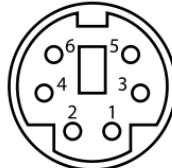
The control system has a purple coloured 6-pin mini-DIN socket (PS2) identified as "KEYB". Any commercially available AT-compatible quality keyboard equipped with the required connector can be connected with this socket. Check the keyboard for proper function before using it.
