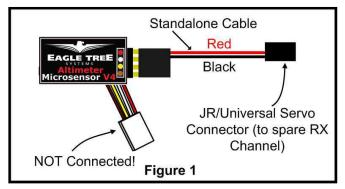
For standalone mode (not connected to an eLogger), connect the Standalone Cable to the gold pins of the Altimeter, as shown in Figure 1. The polarity of the connection is as follows: RED = Positive (Vdd) BLACK = Negative (ground)
