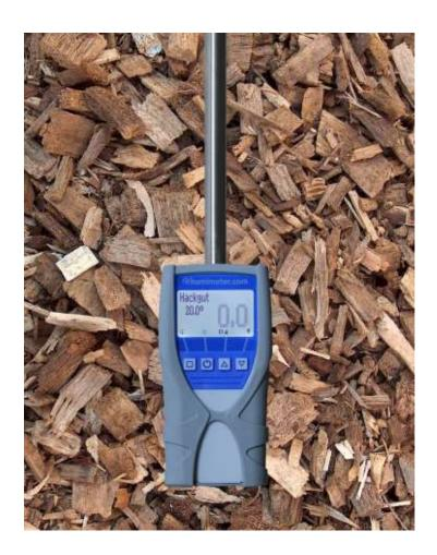
Moisture meter with insertion probe for determination of water content of wood chips
