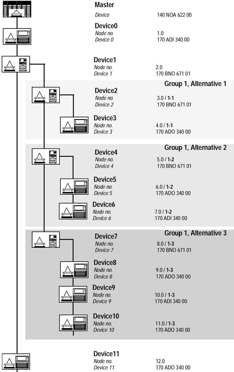
Hardware configuration to INTERBUS network with alternatives
