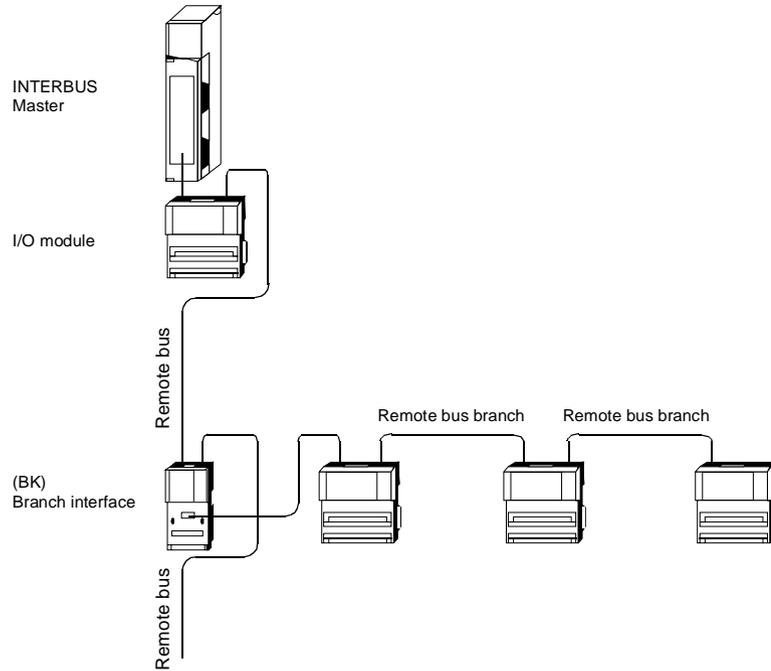
**Note:** With INTERBUS Firmware Generation 4, it is possible to create branches ("branch in branch"), also see picture *INTERBUS architecture*, p. 16.
