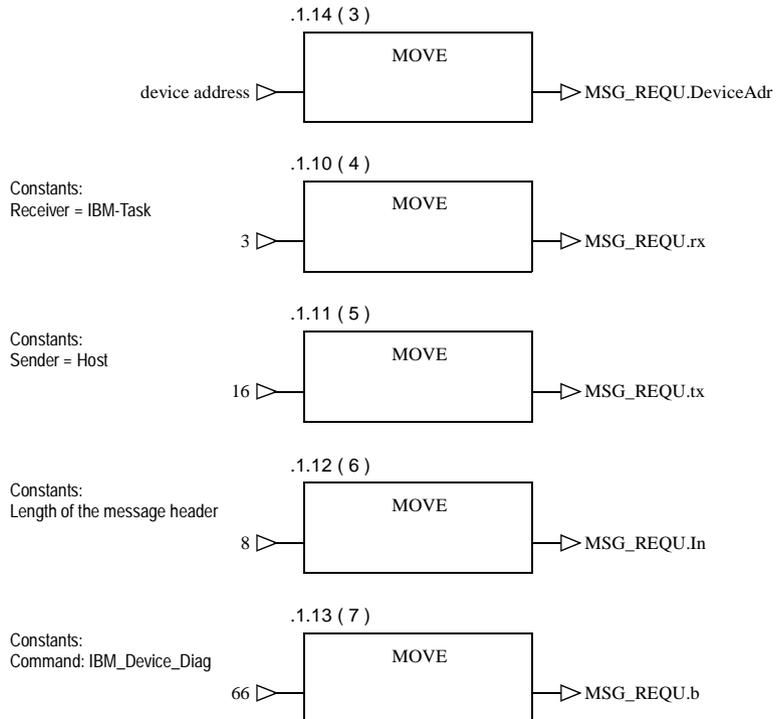
Call for EFBs IBS\_SEND\_REQ to get the diagnosis data from the desired node address:
