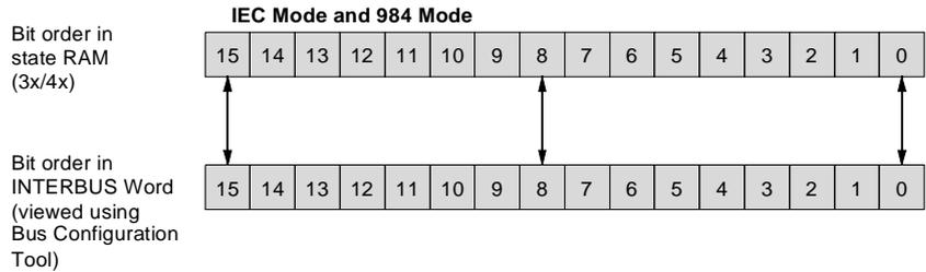
**Binary 8 Bit I/O Module (in 0x/1x and 3x/4x Range)**
