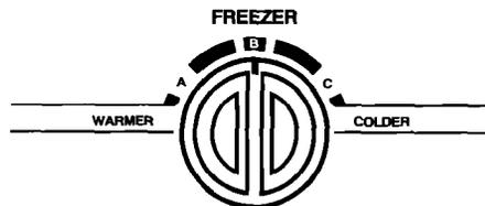
The settings indicated above should be correct for normal, household refrigerator usage. The controls will be set correctly when milk or juice is as cold as you like and when ice cream is firm. If you need to adjust these settings, see "Changing the control settings" on page 8.
