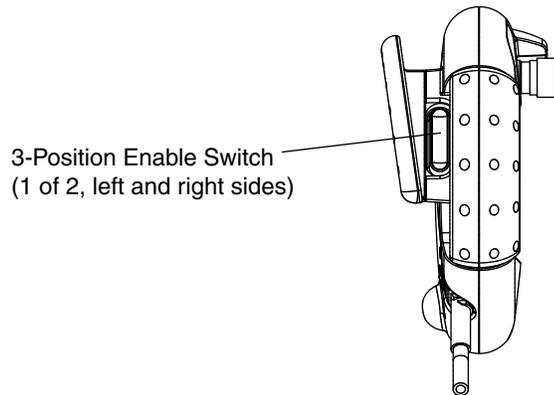
The actuating element consists of two symmetrically arranged slides. The position of these slides is detected by electrical switches and transmitted to the evaluation electronics.
