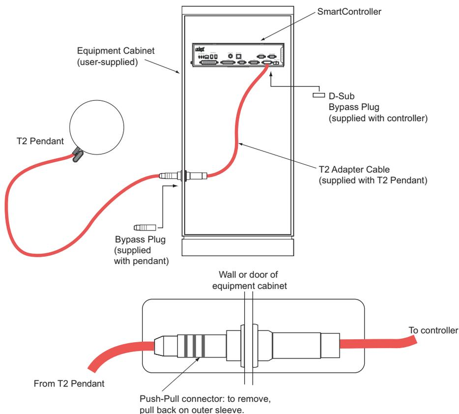
**Figure 2-1. Installing Pendant in Equipment Cabinet**
