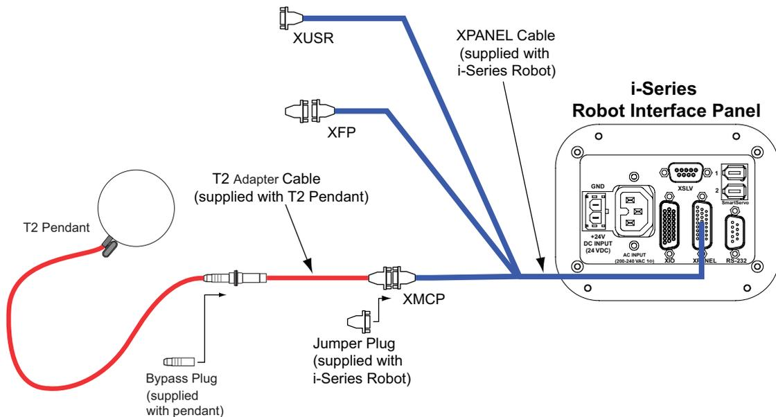
Figure 2-3. Installing Pendant in a Cobra i-Series System
