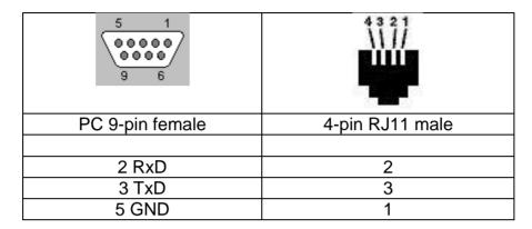
The following wiring diagram can be used to connect computer's RS-232 serial port and JAZZ PLC communication interface:
