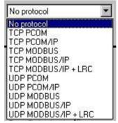
**TCP PCOM** – Unitronics PCOM ASCII serial protocol (encapsulated) over TCP/IP Ethernet. The TCP messages contain pure serial PCOM commands. The protocol implies that at PLC side the TCP/serial conversion is performed (e.g. by GPRS-modem
