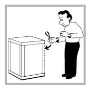
2. Lift off the polystyrene top cap and remove the four corner posts.
