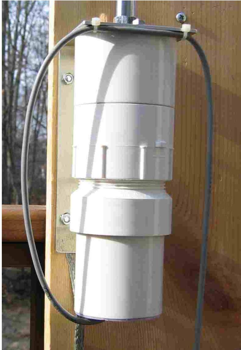
The Model GI-100/1000 is a professional quality, low distortion AM transmitter unit that is designed for continuous outdoor use. It is FCC certified to operate in the standard AM broadcast band and can be operated unlicensed in accordance with Part 15 of the FCC code. Made in USA.
