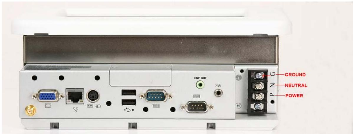
Figure 1.1 I/O Ports
