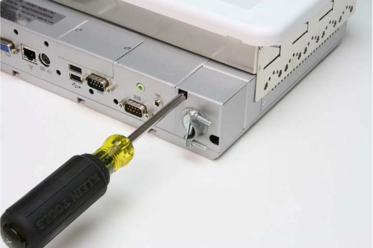
Figure 2 Use access holes to release screws.
