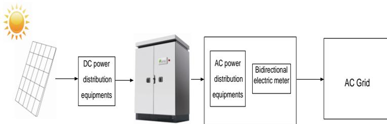
Figure 2-1 Grid-tied PV system
