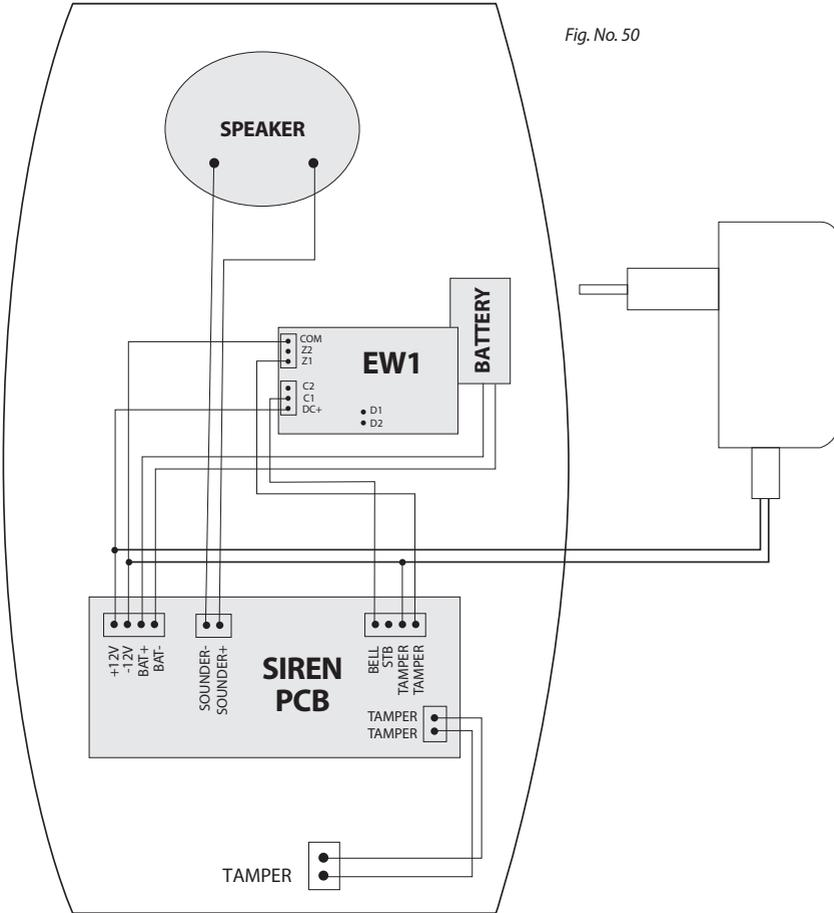
1. Connect the power supply and battery cables as shown in diagram (see Fig. No. 50).
