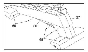
Next, remove the indicated M5 x 25mm Screw (93) and M4 x 16mm Screws (57) from the Right Side Shield (27). Using an adjustable wrench, turn the Right Pedal (21) counterclockwise and remove it. Turn the Right Crank Arm (23) so that it is pointing toward the front of the exercise cycle, and then slide off the Right Side Shield.
