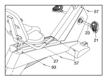
Locate the Reed Switch (46). Turn the Right Crank Arm (23) until the Magnet (30) is aligned with the Reed Switch. Loosen, but do not remove, the indicated M4 x 16mm Screw (57). Slide the Reed Switch slightly closer to or away from the Magnet. Then, retighten the Screw. Turn the Right Crank Arm for a moment. Repeat until the console displays correct feedback. When the Reed Switch is correctly adjusted, reattach the Right Side Shield (27) and the Right Pedal (21).
