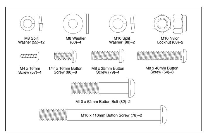
Identify the Front Stabiliser (15). Whilst another person lifts the front of the Frame (1), attach the Front Stabiliser to the Frame with four M8 x 40mm Button Screws (54) and four M8 Split Washers (55).
