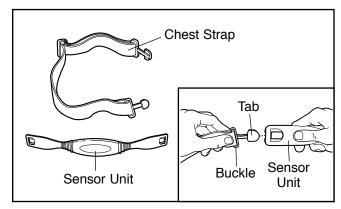
See the inset drawing above. Insert the tab on 1 one end of the chest strap through one end of the sensor unit. Press the end of the sensor unit under the buckle on the chest strap.
