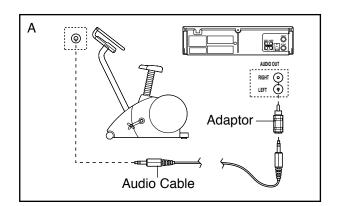
B. Plug one end of the audio cable into the jack beneath the console. Plug the other end of the audio cable into the adaptor. Plug the adaptor into an RCA Y-adaptor (available at electronics stores). Next, remove the wire that is currently plugged into the AUDIO OUT jack on your VCR and plug the wire into the unused side of the Y-adaptor. Plug the Y-adaptor into the AUDIO OUT jack on your VCR.
