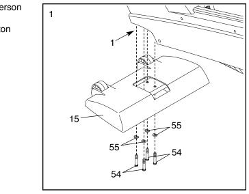
Whilst another person lifts the rear of the Frame (1), attach the Rear Stabiliser (16) to the Frame with four M8 x 40mm Button Screws (54) and four M8 Split Washers (55).
