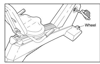
If the exercise cycle rocks slightly during use, turn the leveling feet under the rear stabiliser until the rocking motion is eliminated.
