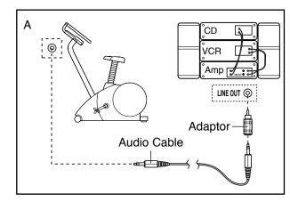
B. Plug one end of the audio cable into the jack beneath the console. Plug the other end of the audio cable into the adaptor. Plug the adaptor into an RCA Y-adaptor (available at electronics stores). Next, remove the wire that is currently plugged into the LINE OUT jack on your stereo and plug the wire into the unused side of the Y-adaptor. Plug the Y-adaptor into the LINE OUT jack on your stereo.
