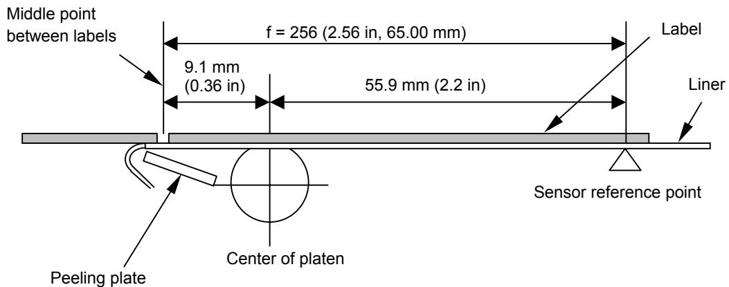
**Note:** If the printer setting (Native ON/OFF) is Native OFF, the reference point (the distance to the print head) will change to 27.9 mm (1.10 in). Therefore, the initial value of the feeding amount to the peeling position will change to:
