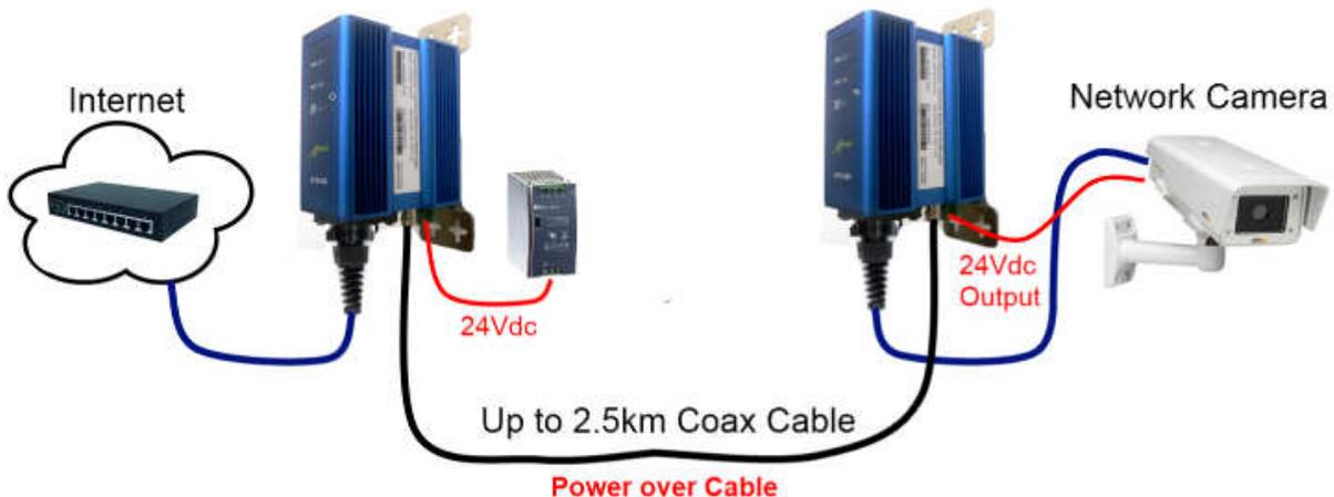
At this point, the essential deployment is completed. Other network segments/devices should be able to communicate with each other via coax link. You may want to configure those APS3400-200s settings by using the Ultra NetBridge™ Utility or via web configuration described by the next two chapters.
