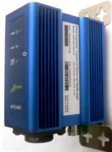
The Aboundi APS3400-200-04 UltraSpeed™ CoaxLine Ethernet NetBridge™ enables the efficient networking deployment utilizing the existing coaxial cable wiring infrastructure already in place. It provides a reliable high speed Ethernet connection cost effectively without the folk lift upgrade for any high speed IP based networking applications.
