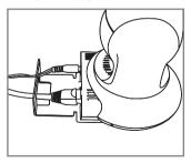
8 Adjust the camera position onto the mounting bracket and tighten the safety screw (A).
