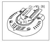
3 Determine the installation place of the camera and mark the places where holes will be drilled on the wall by using the mounting kit.
