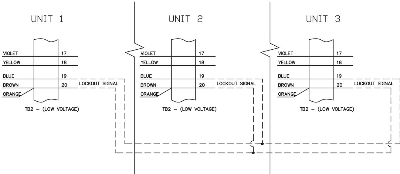
Figure 2 Parallel/Interlock Connections
