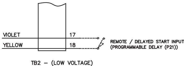
Figure 6 Remote Regeneration Start Connections
