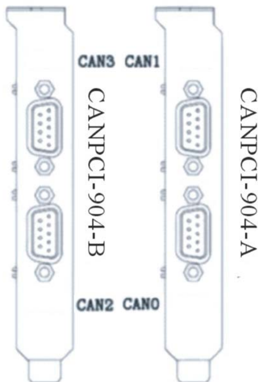
Fig. 2 The CAN channel defined sequence
