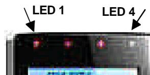
The IQ Standard LCD Terminal has 4 LED indicators which can be used to provide Area status information. Each LED can be programmed to indicate AREA Armed (LED on) and Area in Alarm (LED flashing). Any of the 4 Areas (8 Areas in the IQ Plus System) can be chosen for display.
