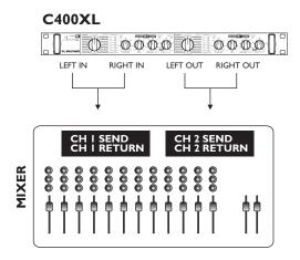
In this example the C400XL is used in Dual Mono mode as two 100% independent mono engines on two separate channels. The two engines have no influence on each other.
