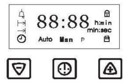
Touchpad SET(-): Conductive key fitted into Touchpad position 1 or 2 Touchpad SELECT: Conductive key fitted into Touchpad position 3 Touchpad SET(+):Conductive key fitted into Touchpad position 4 or 5
