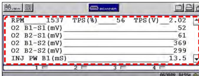
Figure 4-7 Sample Scanner main body
