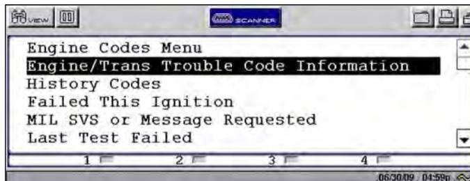
Figure 5-8 Sample Trouble Codes submenu
