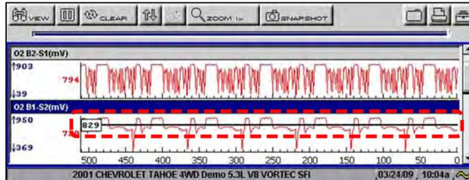
**Figure 5-26** Sample active trigger line
