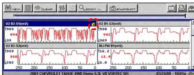
Figure 5-24 Lock icon indicating a locked parameter
