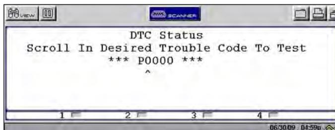
Figure 5-9 Sample DTC Status entry screen
