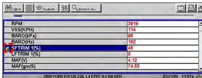
Figure 5-20 Locked PID sample
