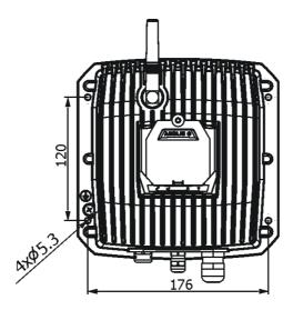
Four holes with diameter of 5.3mm in the control unit are intended for mounting on a flat, non-flammable surface. The length of the connection cable between the ArcPower 48 Outdoor US and the LED unit should not exceed 20 m.
