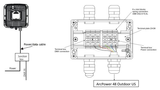
Connect the junction box to mains and DMX acording to the tables below
