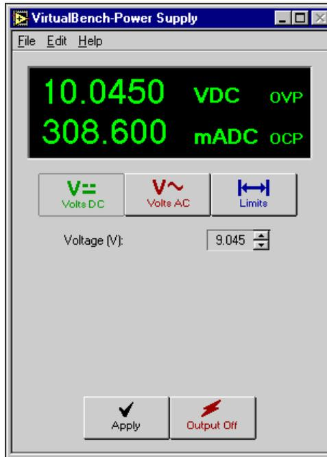
Figure 7-3. Front Panel with Volts DC Button Selected
