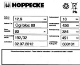
Fig. 1-1: Example for type plate on battery rack
