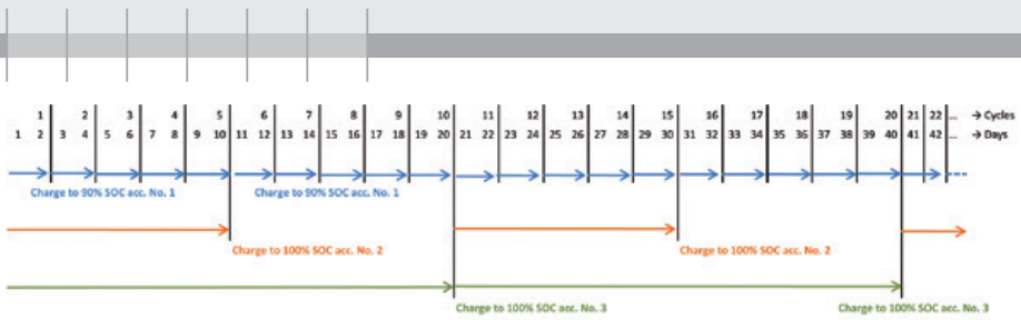
Fig. 7-5: Battery cycles ranging longer than one day
