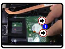
4. Press down on the rubber case 2 to ensure the assembly is properly seated before replacing the cover and screws.
