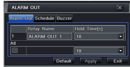
Fig 4-28 system configuration-alarm out
