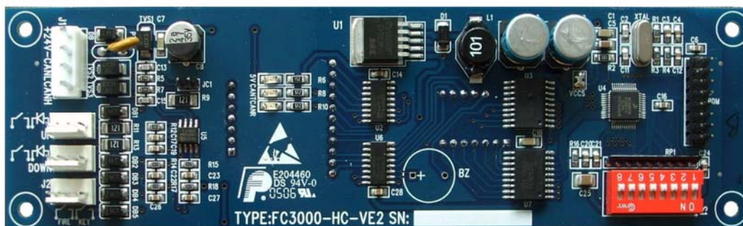
Picture 7 : hall call control device HC_VE2 (Components side)
