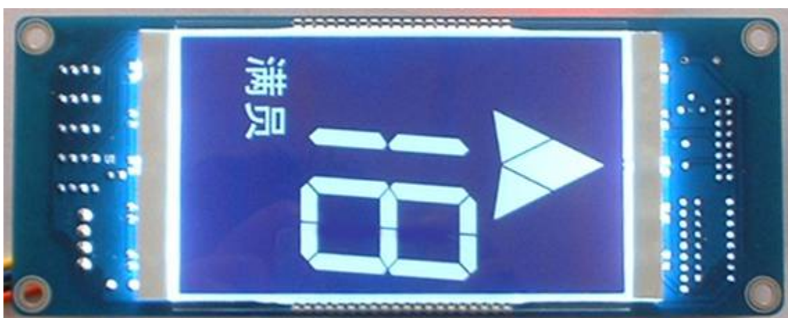
Picture 12 : hall call control device HC_LCD_MI (Displaying side)
