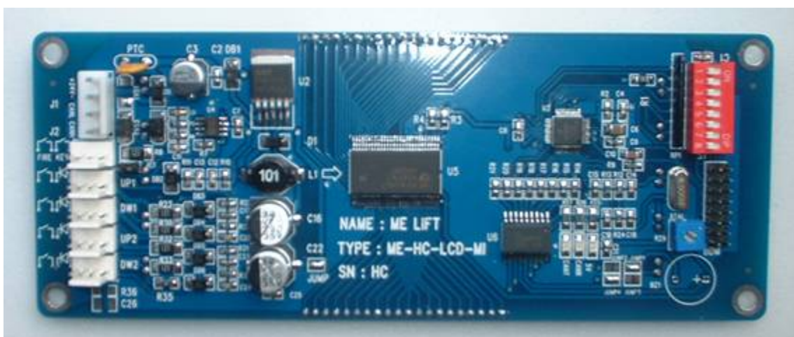
Picture 12 : hall call control device HC_LCD_MI (Displaying side)
