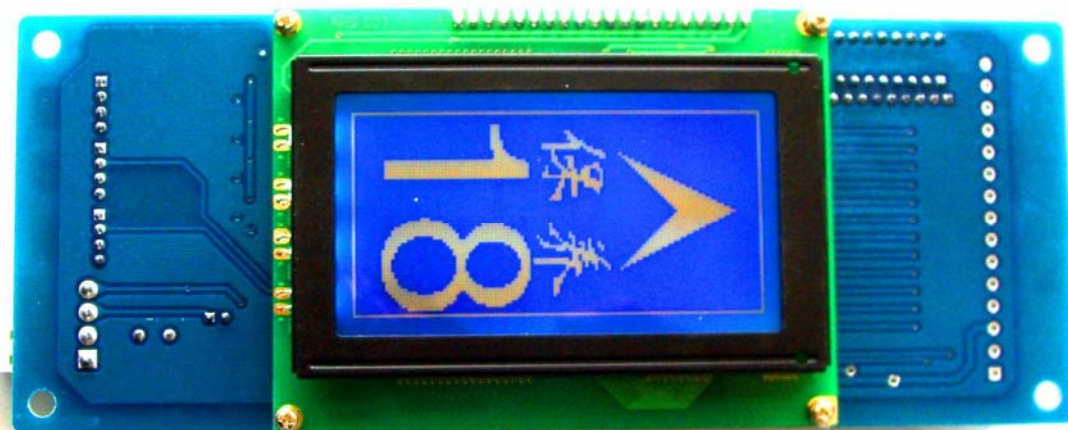
Picture 8 : hall call control device HC_VE3 (Displaying side)
