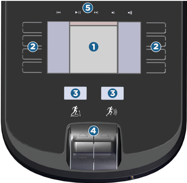
Figure 9: Controls and display areas
