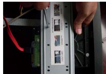
③fix the screw of hard disk
