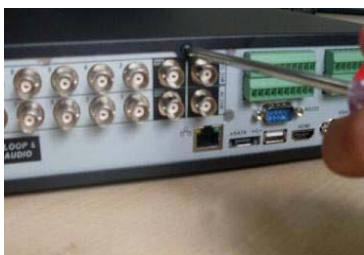
①disassemble the screw
