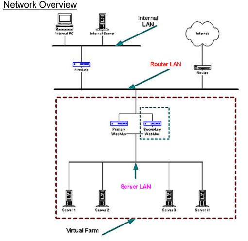
The main purpose of the WebMux is to balance the traffic among multiple web or other servers. The diagram above shows an installation with two WebMuxes. In this configuration, one WebMux serving as the primary, and the other serving as the secondary, or backup, provides a fault tolerant solution.
