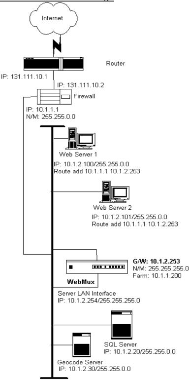
The above diagram is an example about how to install the WebMux without changing the IP addresses of the web servers and other servers that already exist on the network. This is particularly helpful when changing existing network
